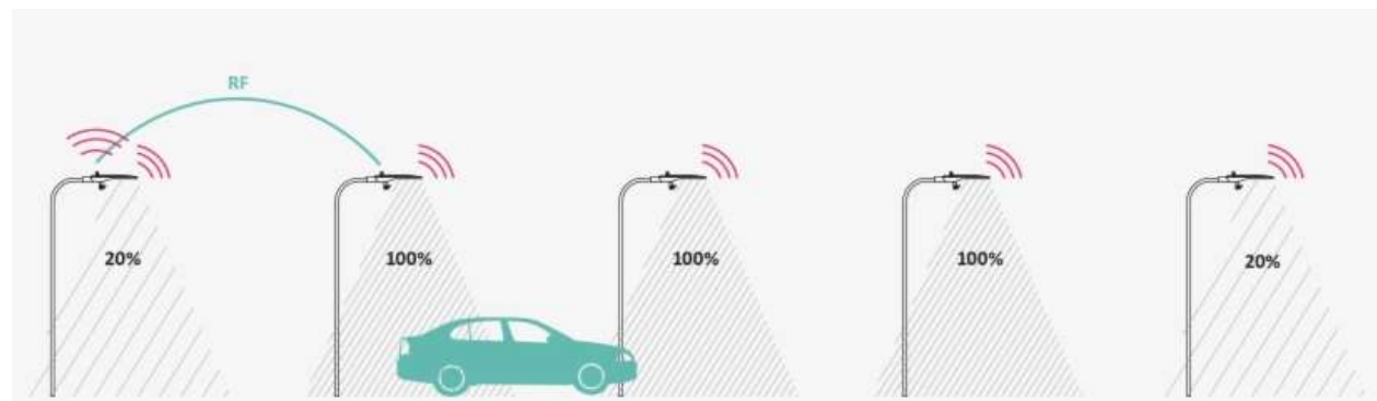
Figure 4 Motion Sensor Street Lighting Control System Illustration
